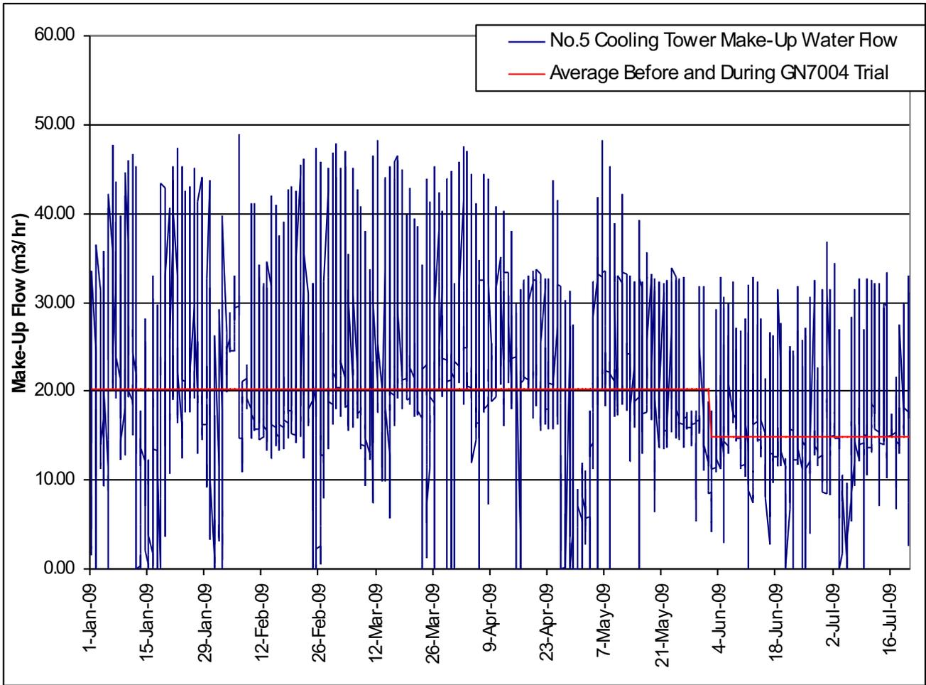
Water consumption improved greatly, as well, because GenGard allowed the tower cycles to be raised from 4.5 to 9 cycles. Figure 2 shows the makeup water flow rate taken from the plant control and monitoring system every hour. Using GenGard GN7004 resulted in an average water consumption savings of 5.33m<sup>3</sup>/hr, which translates into an annual savings of \$42,000.
